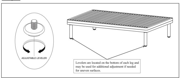
Assembly is now complete and the product is ready for use. Adjustable levelers are located on the bottom of each leg and may be adjusted by turning outwards, counter-clockwise to help account for uneven surfaces. NOTE: Hardware may loosen over time. Periodically check that all connections remain tight and adjust as needed.
