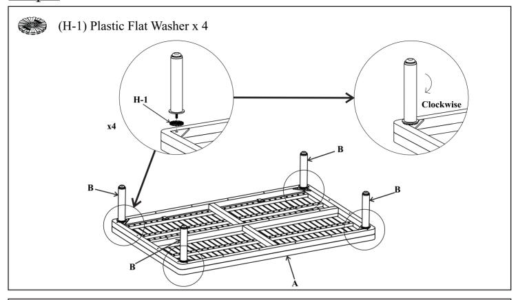
Using a second person to assist you, place Tabletop (A) upside down onto a padded, non-marring surface. Position the Legs (B) on Tabletop (A) as shown. Position the Plastic Flat Washers (H-1) between the legs and the Tabletop (A) and tighten by turning clockwise. DO NOT OVER TIGHTEN.
